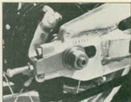
Answer Products makes this weld-on extension for the 250 swingarm which adds an extra inch of wheelbase to the rear end.
