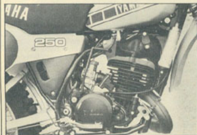
New exhaust pipe has an enormous head and belly section. It could use a heat shield to prevent leg burns.
