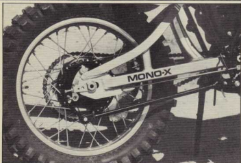
This will probably be the last year you'll see the traditional Yamaha Monoshock design. The factories are playing with a progressive setup similar to the Honda Pro-Links.
