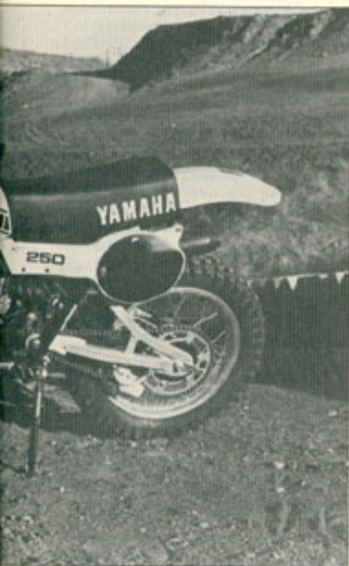
Peering under the rear fender, one can see aluminum fins on the rear of the monoshock unit.
