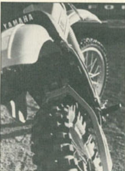
Peering under the rear fender, one can see aluminum fins on the rear of the monoshock unit.
